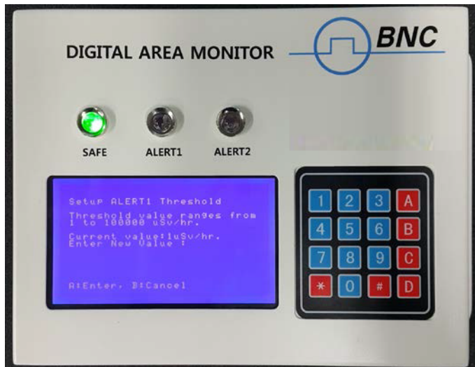
Figure 10. setup alarm threshold example (ALERT1 case)
